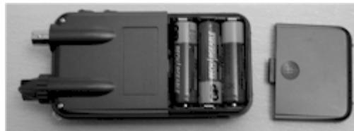
Power requirement: TRX-200 can be operated from either three AA size Ni-Cad. batteries, three AA size dry cell batteries or external DC supply of 9 to 14V DC, 300mA minimum.
