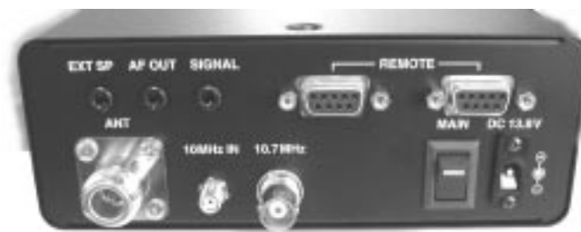
Main Power Switch ___ | ___ DC Power Jack
